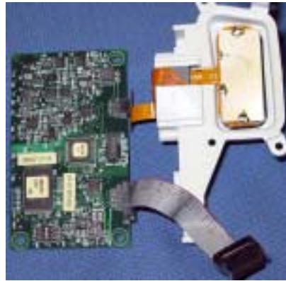
2 screws securing the SpO 2 board to the SpO 2 assembly
