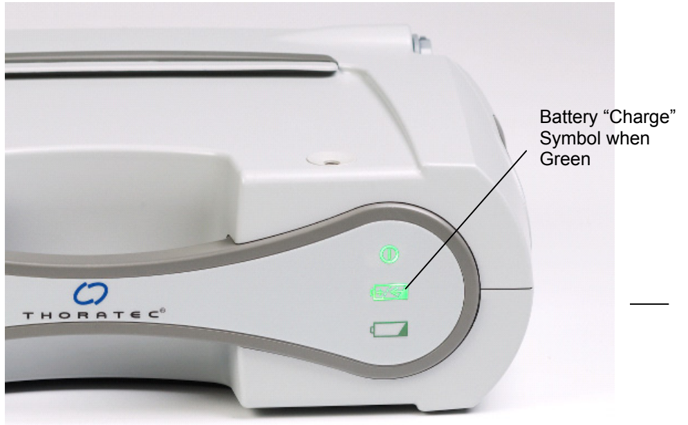
Figure 33 Green Charge Symbol (Internal Backup Battery Ready for Use)
