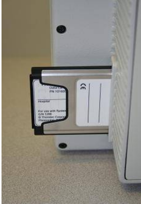
Figure 116 Inserting Data Card into PC Card Adapter inside System Monitor
