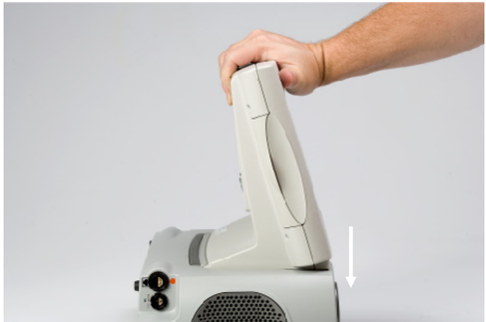
Figure 47 Pressing Down on front of System Monitor to insert Feet into Holding Grommets of the PM
