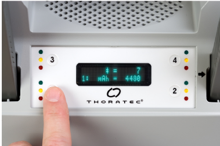
Figure 66 Pressing the Button a Second Time Reveals the Charge/Use Cycle Count (in this case 7 cycles) and the Charge Capacity (in mAh) for the battery (in this case, the battery in pocket #1)
