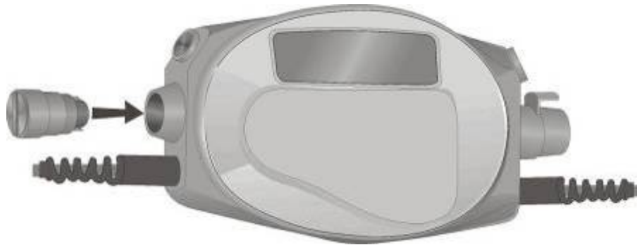
Figure 12 Changing System Controller Battery Module
