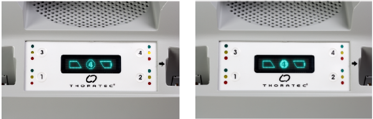
Figure 68 Calibration prompt (in Graphics mode). In this case, the battery in pocket #4 needs calibration.
