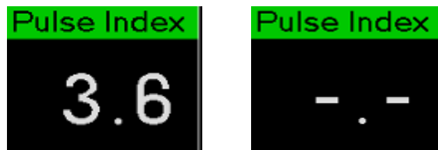
Figure 80 Pulsatility Index under Normal Conditions (left) and When the Pump is Stopped or Disconnected (right)
