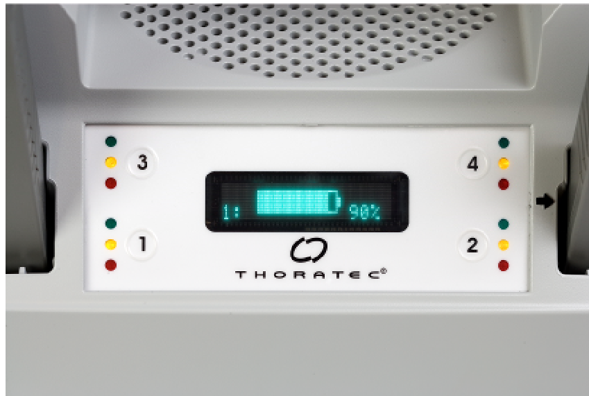
Figure 65 Viewing Available Power for the Battery in Pocket #1 (in Graphics mode). In this case, the battery is approximately 90% charged.
