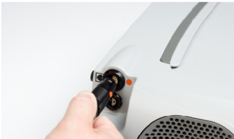
Figure 31 Lining Up Red Dots and Inserting Cable into Socket
