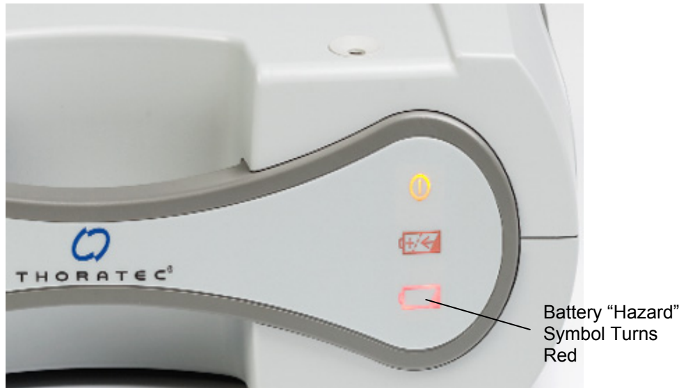
Figure 36 Red Battery "Hazard" Symbol (Less than 5 Minutes of Backup Power Remain) Switch IMMEDIATELY to Another Power Source
