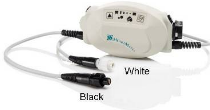
Figure 5 System Controller and Power Leads
