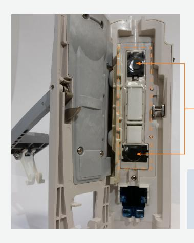
The two pressure sensors are covered by a clear, rectangular membrane shown in the picture at left.
