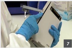
Fully inspect the instrument during each cleaning. Look for any visible external damage, such as a cracked or broken door, handle or latch. Open the door of each pump module, and inspect the platen and hinge for cracks or other damage.
