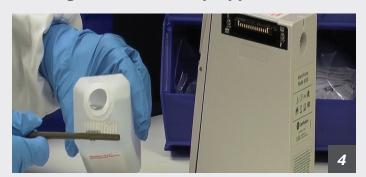
Apply 70% IPA directly to the dedicated IUI cleaning brush. To prevent cross-contamination, do not dip the brush into the IPA.
