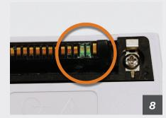
Inspect the IUI connectors on each Alaris PC unit and module prior to use. Replace any IUI connector with surface contaminants, blue or green deposits, damaged contacts, ribs or cracks.
