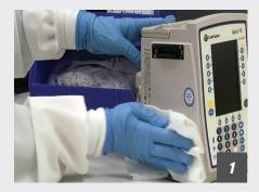
Make sure the instrument is upright and turned off, unplug the power cord and wipe all exposed device surfaces **EXCEPT** the inter-unit interface (IUI) connectors.
