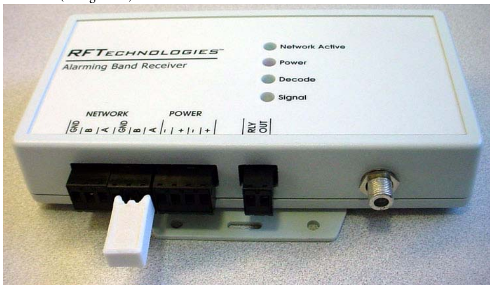
FIGURE 2.2: Resistor termination using a radial 100 ohm resistor
